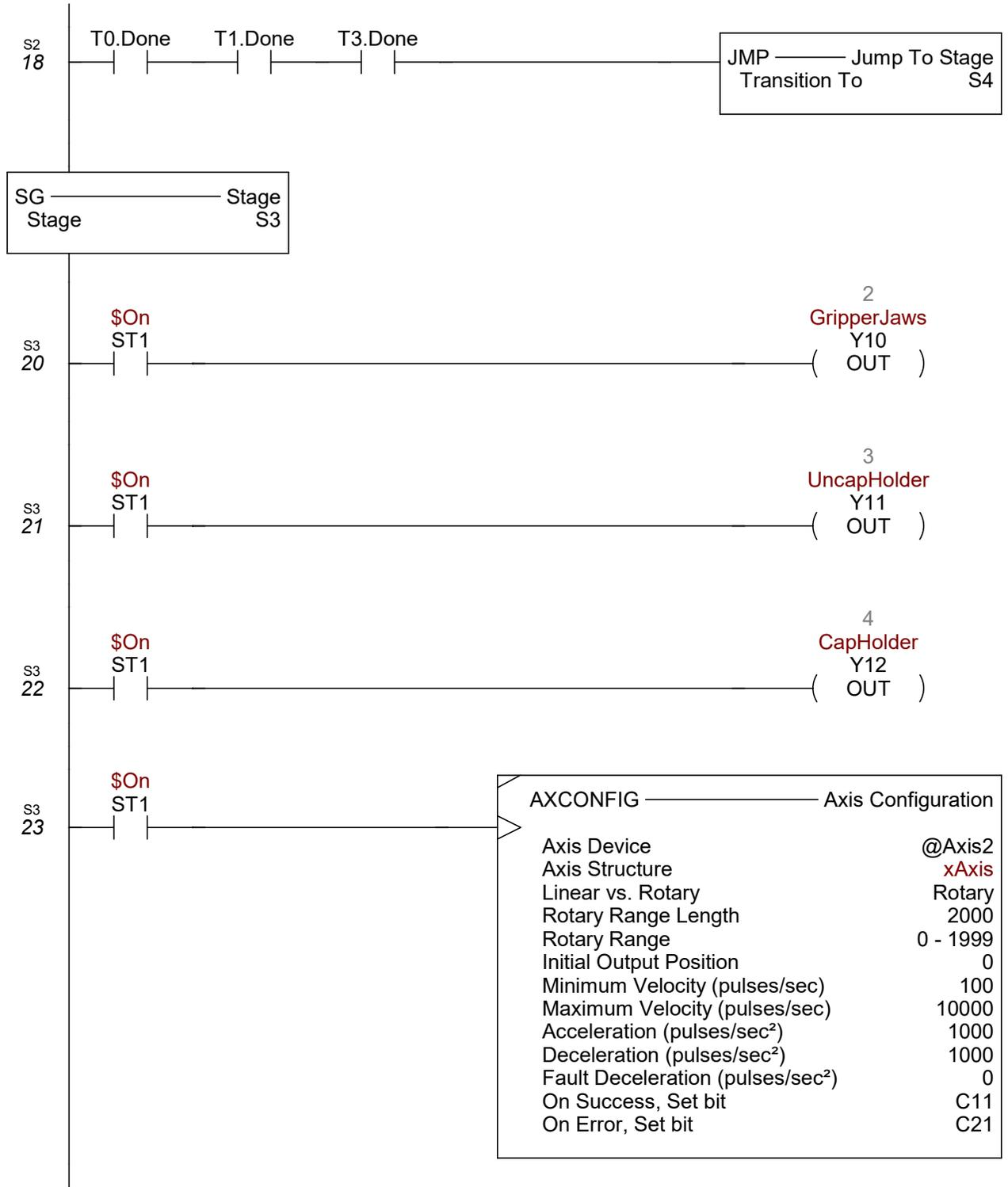
The xAxis will move until the limit switch indicating the capping position has been triggered
