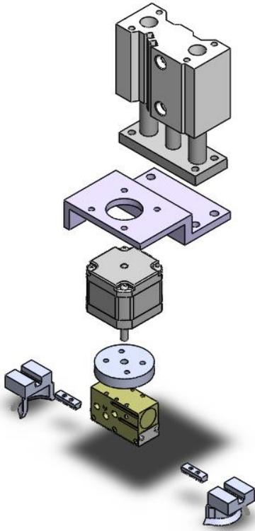
*14 Exploded view of Full Gripper Assembly*
