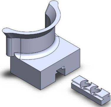
*12 Gripper and Gripper Mount*
