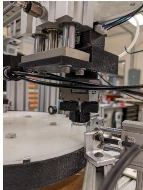
Figure 5: Gripper Head
