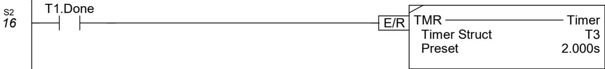
After the jaws are closed and the program has waited for a set amount of time, the gripper will spin for a set amount of time at a set velocity
