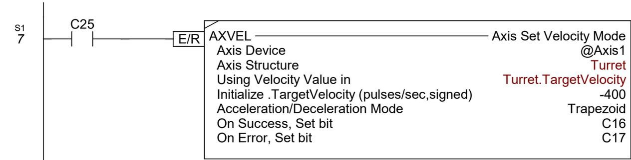
The turret should rotate until the metal strip is sensed to indicate that it is in position
