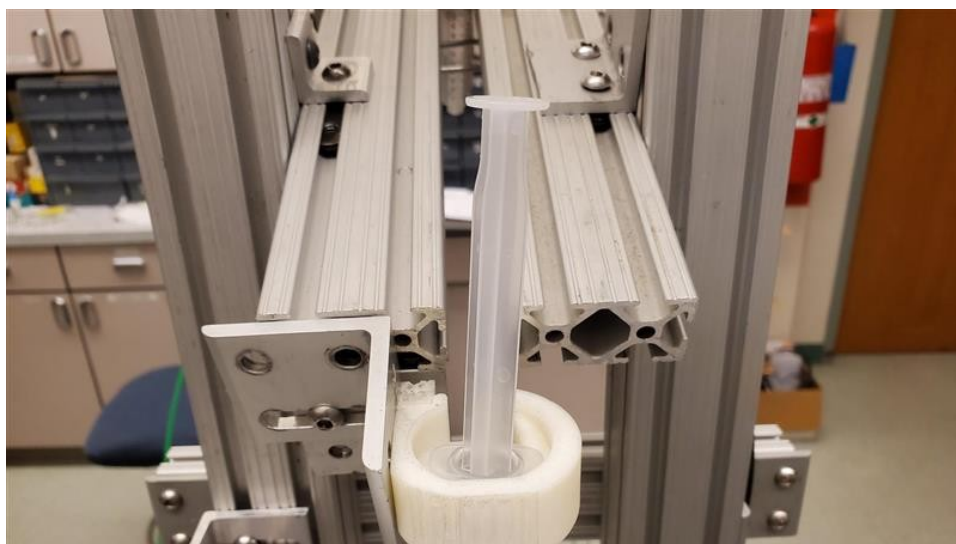
Figure 4: Syringe entering the syringe-orienting chute
