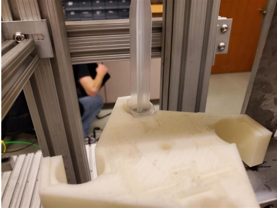
Figure 6: Syringe in the first position of the rotating mechanism
