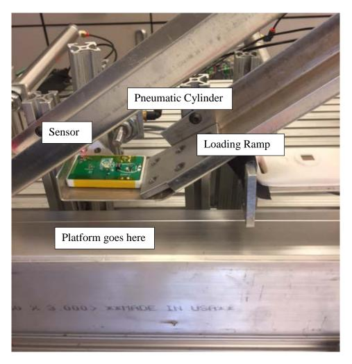
The second stage is almost identical to the first stage. This stage slides the interior electronics package from its loading ramp into the bottom half of the headlamp via a pneumatic cylinder. Just like stage 1, after the optical sensor senses that the part has been moved from the loading ramp, the IAI slide moves the platform to stage 3.
