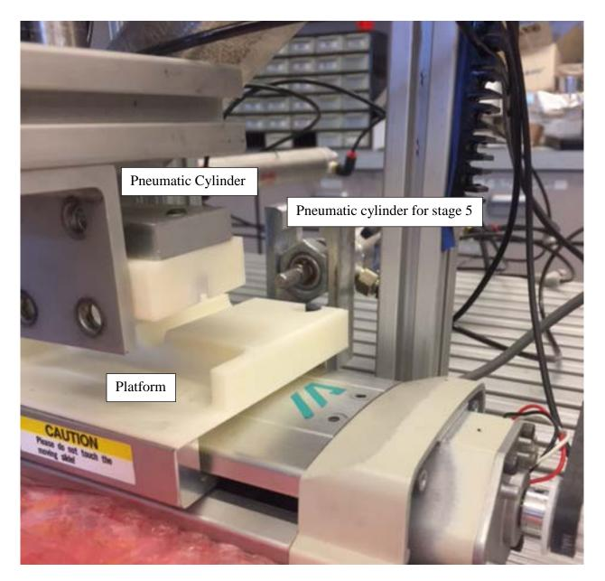
The fourth stage is where the parts get snapped together. A pneumatic cylinder above the assembly line comes down and pushes the two halves of the headlamp together. To do this, the inverse of the top half of the headlamp was 3D printed and then attached to the end of the pneumatic cylinder. The sloped sides of the snapping mechanism also helps to align the parts if they are still slightly off after the alignment process. Two Hall Effect sensors detect when the
