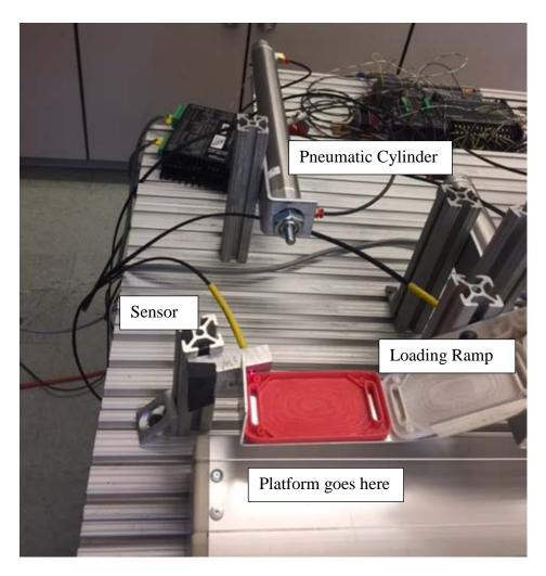
The first stage in the assembly places the bottom half of the headlamp case onto the platform located on the slide. A loading ramp slides the parts down to the level of the assembly line and then a pneumatic cylinder pushes the part from the bottom of the ramp onto the platform. An optical sensor senses when the part has been removed from the assembly line and after a time delay, the slide moves to stage 2.
