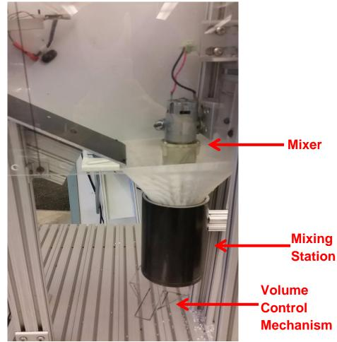
Figure 8. The Mixing Station.
