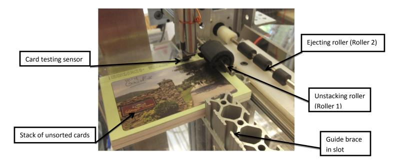
The unstacking roller is not round. It is shown in neutral position so it won't put pressure on the paper while the ejector roller pulls the paper away.
