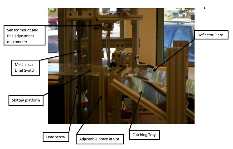
This system is advantageous because it has the potential to be very fast because movement is minimized. The components are relatively cheap because it requires no robotics, pneumatics, or PLC control. The machine also has the potential to process a large stack of paper, limited only by the length of the lead screw. Switching between sizes of paper requires the operator to adjust only one guide rail and the backstop of the catching tray.
