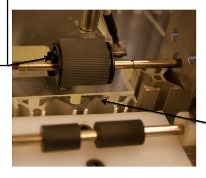
Fixed stop allows one card at a time to pass.
