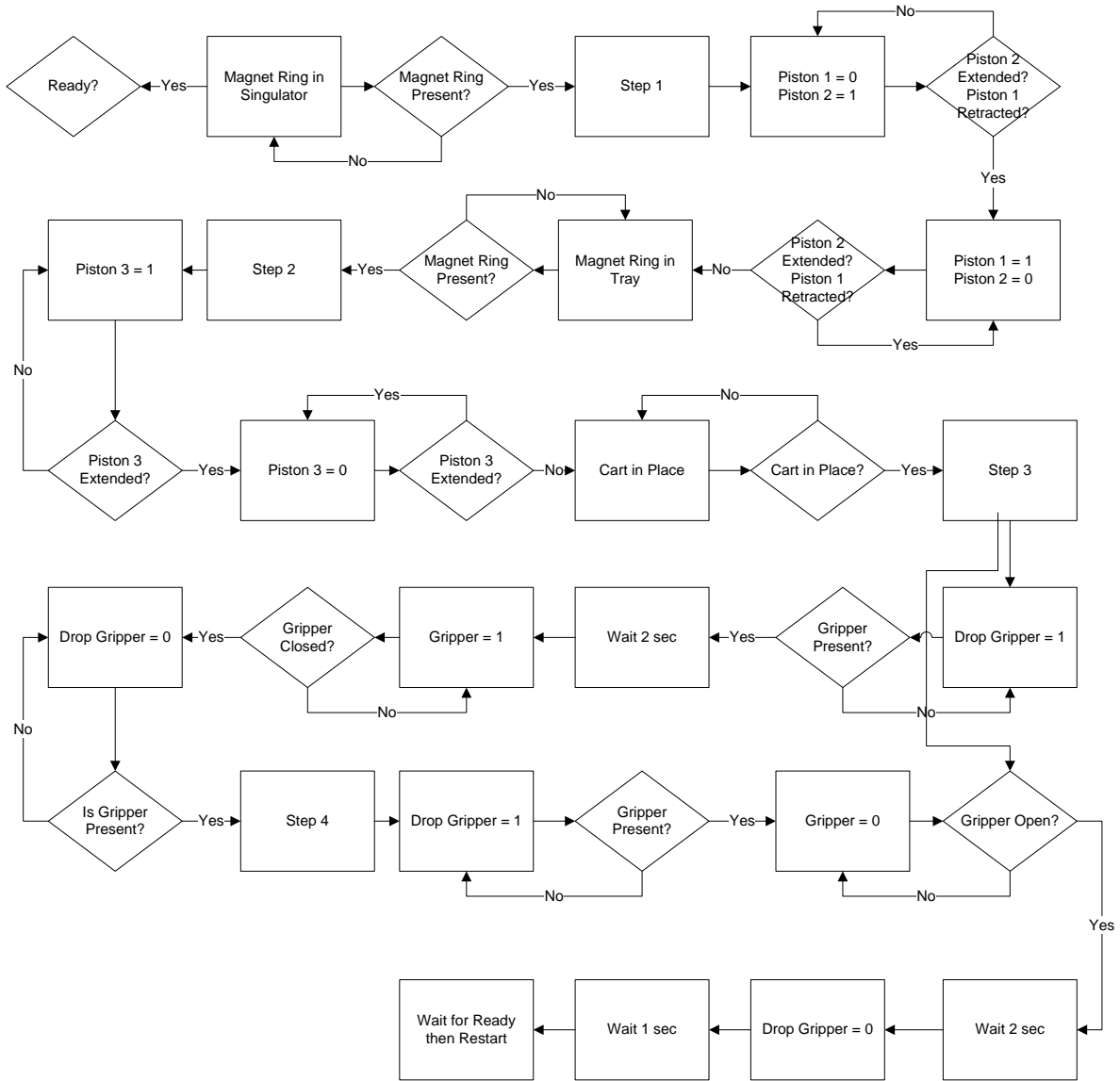
Figure 17: Magnet Ring/Outer O-Ring State Diagram:
