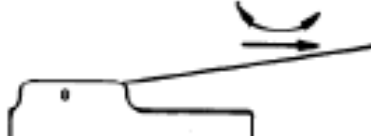
Lever; Very low force, slow cams and slides
