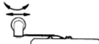
Roller leaf; Low-force, large movement actuation
