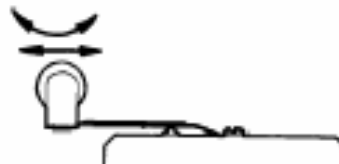
Roller leaf; Low force, large movement actuation
