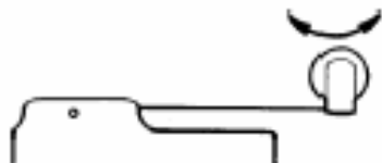
Roller lever; Very low force, fast moving cams
