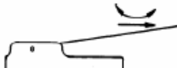
Lever; Very low force, slow cams and slides
