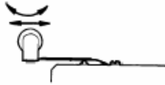
Roller leaf; Low-force, large movement actuation
