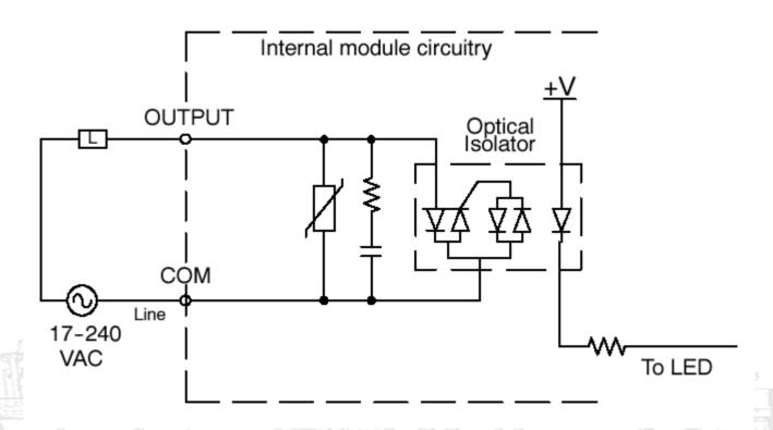
Triac switch turns on or off at AC zero voltage points.
