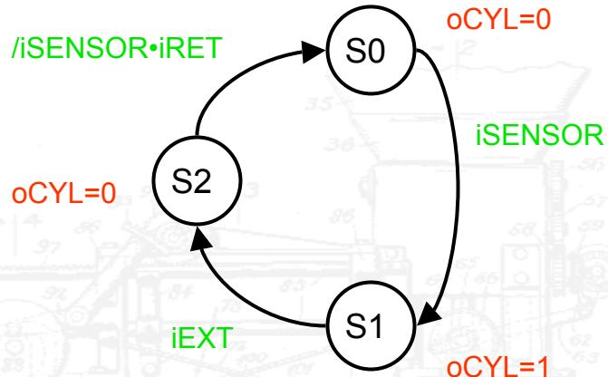
$$cS0 = cS2 \cdot /iSENSOR \cdot iRET + cS0 \cdot iSENSOR + /cS0 \cdot cS1 \cdot /cS2$$
