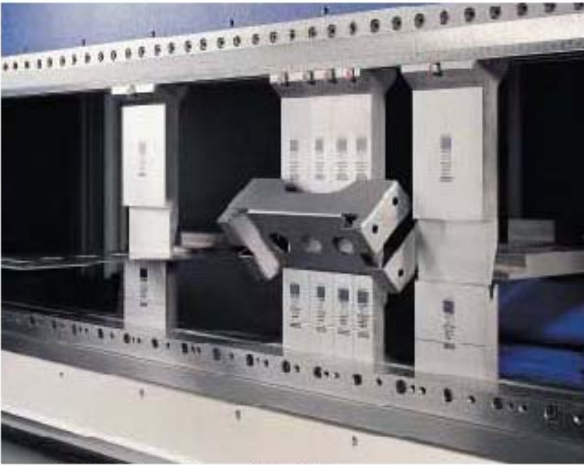
Press brake bending with several tool stations
