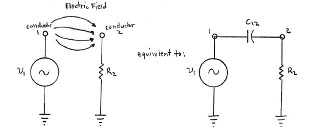
A time-varying voltage on a conductor will create a time-varying electric field. Another nearby conductor intercepting this field will have a corresponding voltage induced on it. This electric field coupling can be modelled as a capacitance between the two conductors. There is also capacitance between each conductor and ground.
