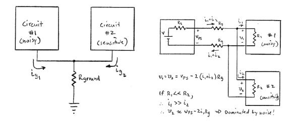
If Circuit #1 has a large dynamic ground current, circuit #2 will see a large dynamic change in the voltage at its "ground" terminal. The solution is to provide separate ground conductors for each circuit all the way back to the common ground point (typically at a power supply), and to reduce R<sub>ground</sub> as much as possible (heavier conductor, better connections).
