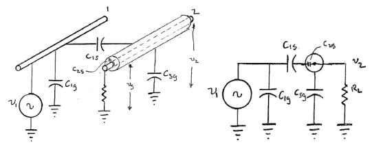
If we ground the shield,  $v_s = 0$ , so  $v_2 = 0$  also! Any portion of the inner conductor that sticks out of the shield will have a small  $C_{12}$  and so will pick up a small noise voltage, but the shield will stop most of the electric field coupling.
