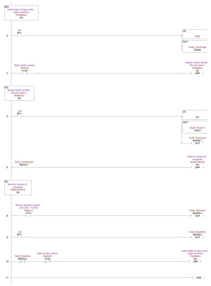
Create PLC logic and step motor motion profile to move when switch0 (X120) is turned on. If switch1 (X121) is off, then the move should be 30 degrees. If X121 is on, then the move should be 120 degrees. Use switch2 (X122) to set the direction of motion.
