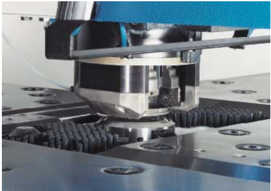
The rotating tool adapter allows all tools to be rotated.
