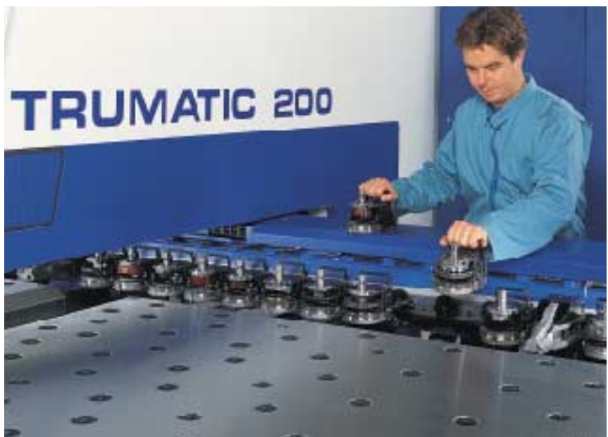
Complete tool sets are set up in the linear magazine.
