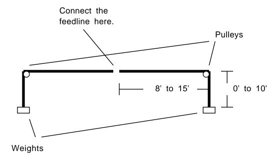
The idea is that the antenna will be able to retract so that the total length will be anything between 16 and 36 feet. It will be retracted normally so that the wind load will be minimum. It will only be extended during use. The features desired are listed below with an importance weighting for each. I have available some sturdy hollow fiberglass poles with the following dimensions:
