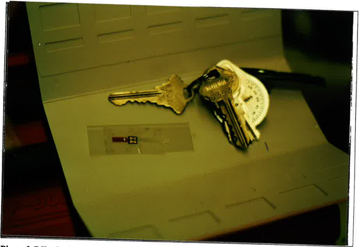
Photo 2.7 Typical Electrical Resistance Strain Gage
