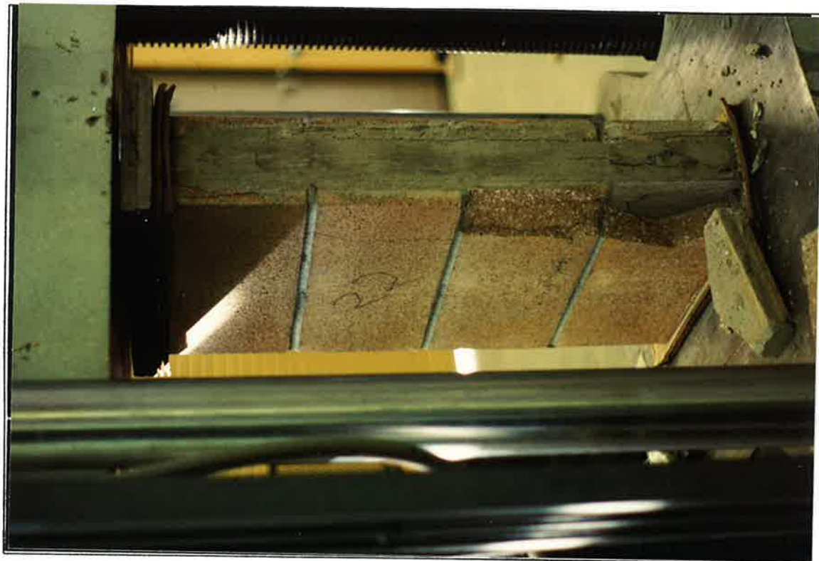
Photo A.3 Masonry Prism Test For Slitted Wall
