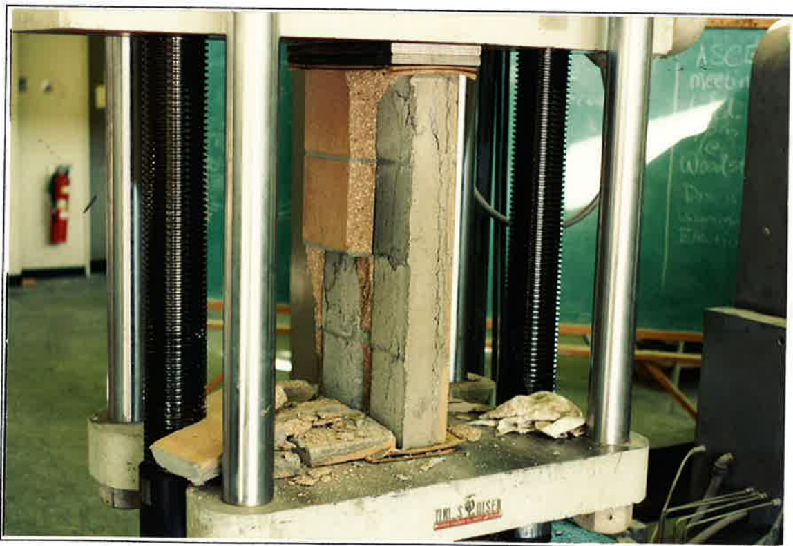
Photo A.4 Masonry Prism At Completion of Compression Test
