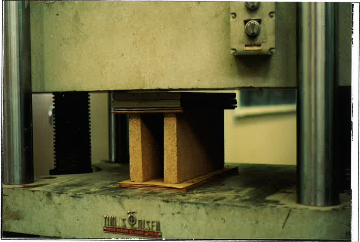
Photo A.1 Compression Test of Typical Open End Bond Beam Unit
