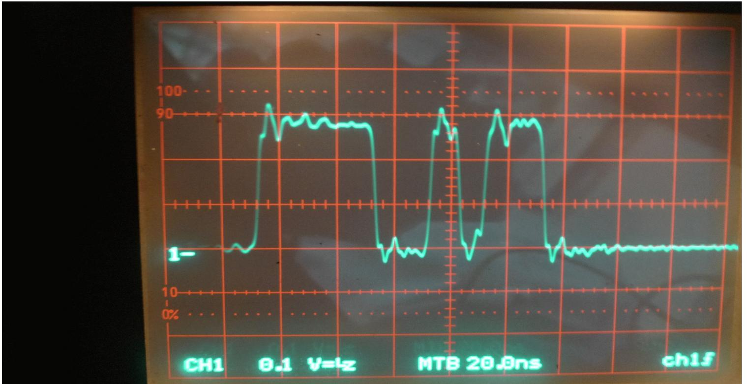
Fluke CombiScope 200 Mhz scope with HP 10020A 10x 500 ohm resistive probe (scope in 50 ohm input mode, and scale is 1V/div)
