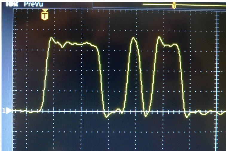
Tektronix TBS2104 100 Mhz scope with factory 10x probe. ~3" long ground lead
