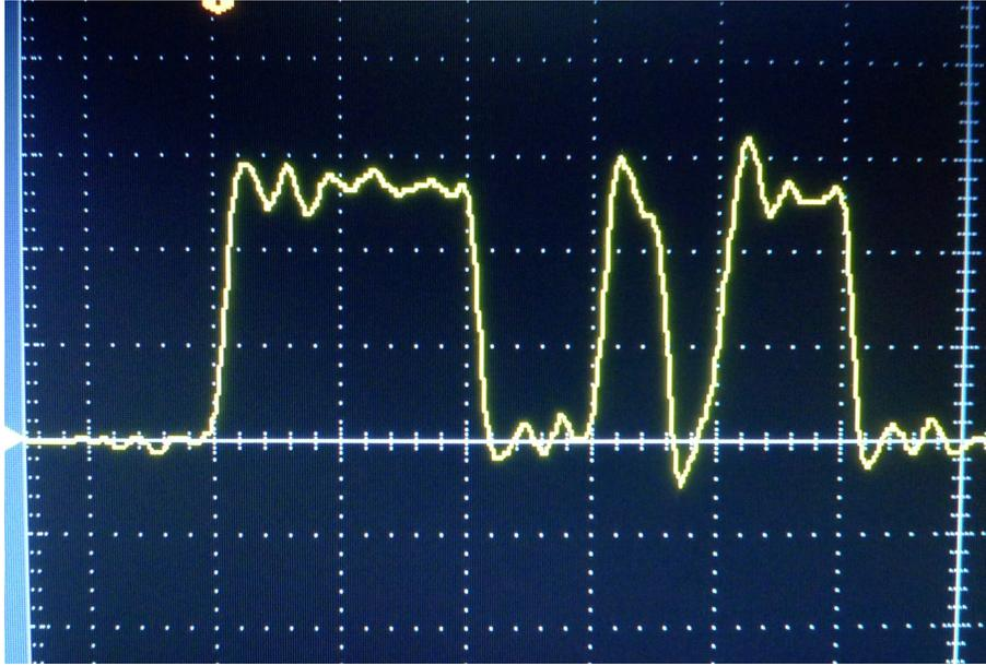
Tektronix TBS2104 100 Mhz scope with HP 10020A 10x 500 ohm resistive probe (50ohm in-line terminator at the scope end of the probe cable)
