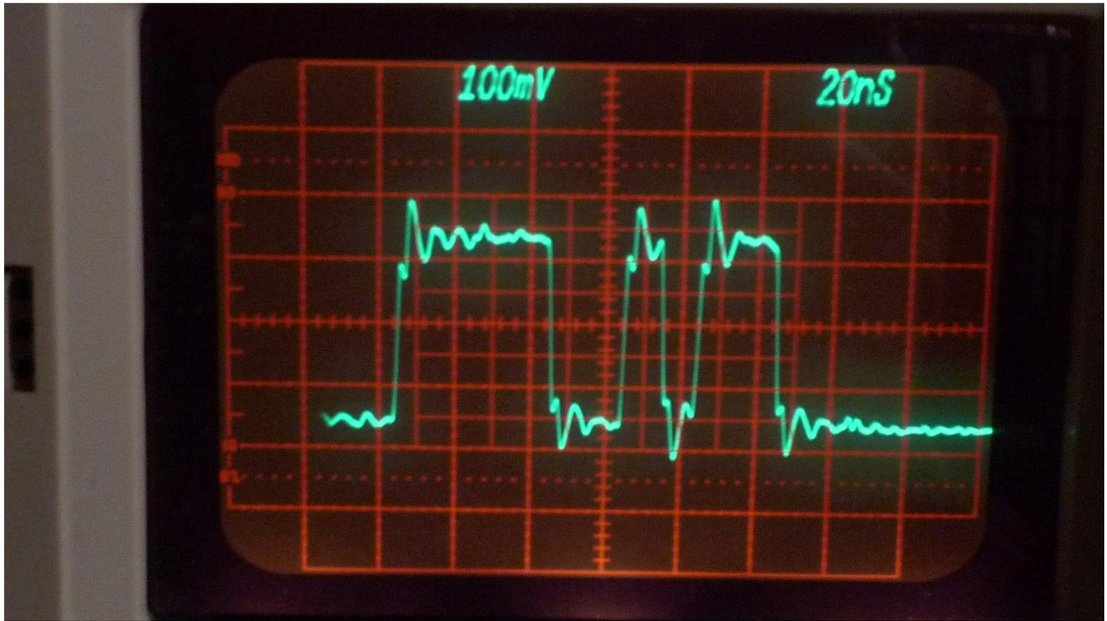
Tektronix 7834 400 Mhz scope, 1GHz vertical amp with 50 ohm input, and a HP 10020A 10x 500 ohm resistive probe (scale is 1V / div).
