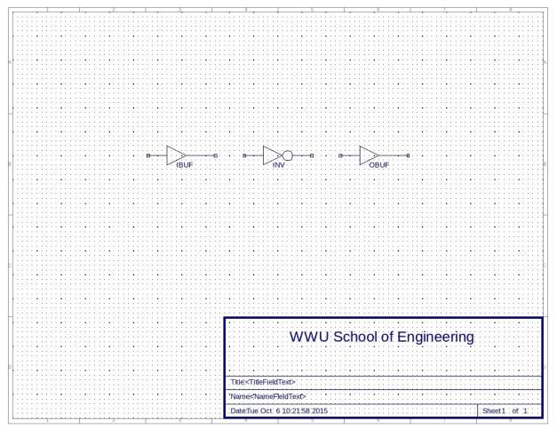
Next the inverter needs to be wired to the input and output buffers.
