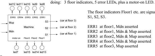
The floor indicators Floor1 etc. are signals S1, S2, S3.
