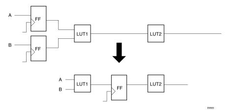
Forward Register Balancing moves a set of flip-flops at the inputs of a LUT to a single flip-flop at its output.
