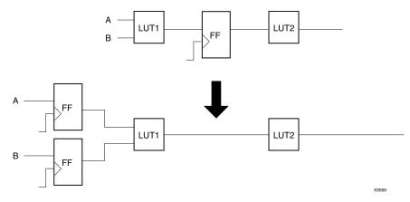
Backward Register Balancing moves a flip-flop at the output of a LUT to a set of flip-flops at its inputs.
