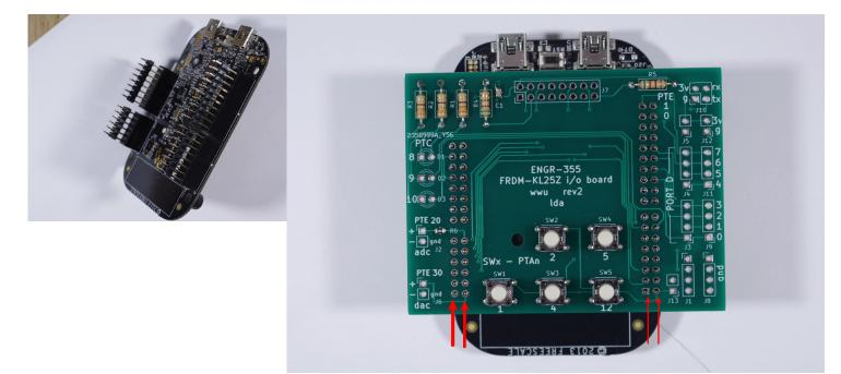
4) Install five male headers. 2-pin for adc and dac; 4-pin for j8, j9, & j11
