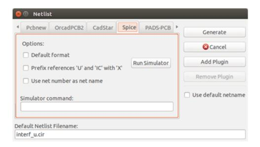
Using the different tabs you can select the desired format. In Spice format you can generate netlists with either equi-potential names (it is more legible) or net numbers (old Spice versions accept numbers only). By clicking the Netlist button, you will be asked for a netlist file name.
