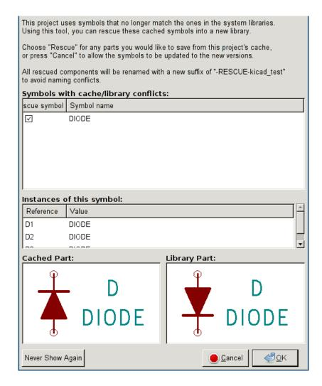
You can see in this example that the project originally used a diode with the cathode facing up, but the library now contains one with the cathode facing down. This change could ruin the project! Pressing OK here will cause the old symbol to be saved into a special "rescue" library, and all the components using that symbol will be renamed to avoid naming conflicts.
