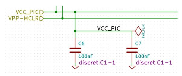
You find again, the two corresponding hierarchical labels, providing connection between the two hierarchical sheets.
