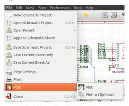
The suported output formats are Postscript, PDF, SVG, DXF and HPGL. You can also directly print to your printer.
