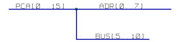
Buses PCA [0..15], ADR [0..7] and BUS [5..10] are connected together (note the junction here because the vertical bus wire joins the middle of the horizontal bus segment).
