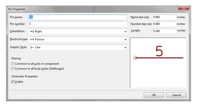
The pin properties dialog allows you to edit all of the characteristics of a pin. This dialog pops up automatically when you create a pin or when double-clicking on an existing pin. This dialog allows you to modify:
