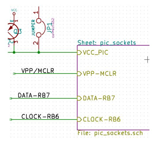
Notice pin VCC\_PIC, connected to connector JP1.
