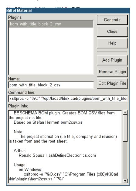
Eeschema's BOM generator makes use of external plugins, generally in XSLT or Python form. Some are provided, and will be installed inside the KiCad program files directory.
