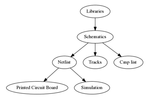
Components are added to the schematic from component libraries. After the schematic is made, a netlist is generated, which is later used to import the set of connections and footprints into PcbNew.
