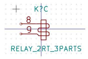
It does not have the same symbol and pin layout and therefore is not interchangeable with units 1 and 2.
