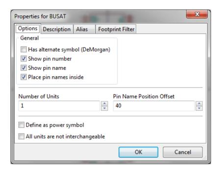
It is very important to correctly set the number of units per package and if the component has an alternate symbolic representation parameters correctly because when pins are edited or created the corresponding pins for each unit will created. If you change the number of units per package after pin creation and editing, there will be additional work introduced to add the new unit pins and symbols. Nevertheless, it is possible to modify these properies at any time.
