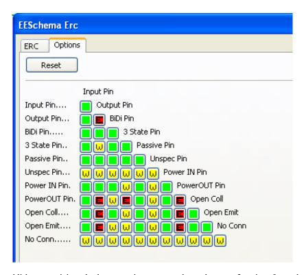
This tab allows you to establish connectivity rules between pins; you can choose between 3 options for each case:
