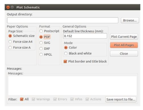
Allows you to create plot files using the format PDF. The file name is the sheet name with an extension .pdf.
