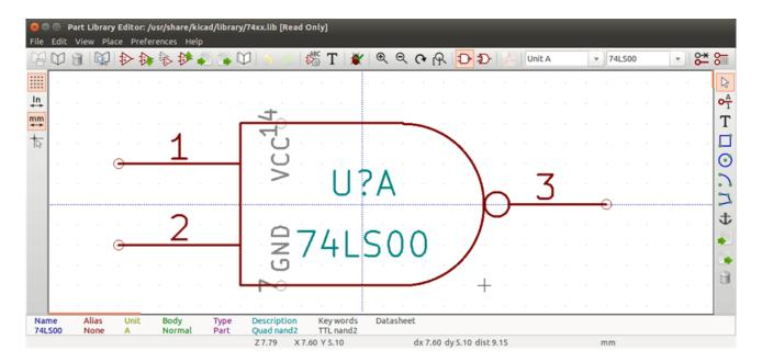
The anchor can be repositioned by selecting the icon and clicking on the new desired anchor position. The drawing will be automatically re-centered on the new anchor point.
