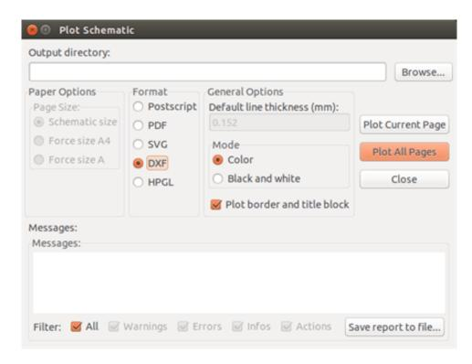
Allows you to create plot files using the format DXF. The file name is the sheet name with an extension .dxf.
