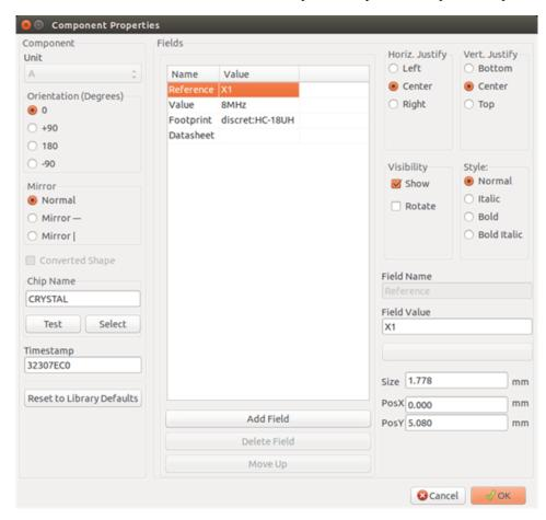
Each field can be visible or hidden, and displayed horizontally or vertically. The displayed position is always indicated for a normally displayed component (no rotation or mirroring) and is relative to the anchor point of the component.
