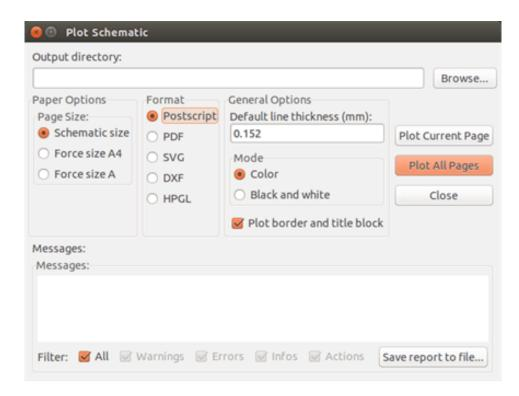
The file name is the sheet name with an extension .ps. You can disable the option "Plot border and title block". This is useful if you want to create a postscript file for encapsulation (format .eps) often used to insert a diagram in a word processing software. The message window displays the file names created.
