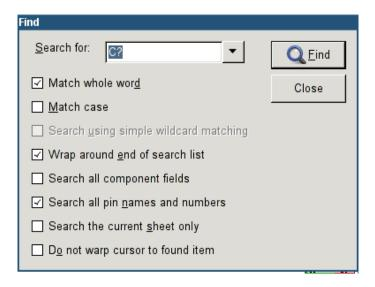
You can search for a reference, a value, or a text string in the current sheet or in the whole hierarchy. Once found, the cursor will be positioned on the found element in the relevant sub-sheet.
