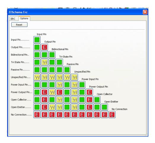
Rules can be changed by clicking on the desired square of the matrix, causing it to cycle through the choices: normal, warning, error.
