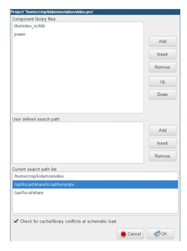
This dialog is used to configure component libraries and search paths. The configuration parameters are saved in the .pro file. Different configuration files in different directories are also possible.
