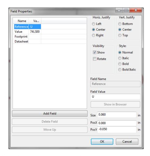
Fields are text sections associated with the component. Do not confuse them with the text belonging to the graphic representation of this component.
