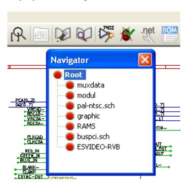
Each sheet is reachable by clicking on its name. For quick access, right click on a sheet name, and choose to Enter Sheet.
