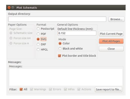
Allows you to create plot files using the vectored format SVG. The file name is the sheet name with an extension .svg.
