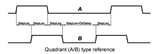
Figure 27.5: Reference signal timing diagrams
