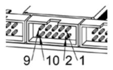
Figure 27.2: Pin numbering of GPIO connectors
