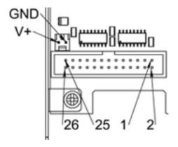
Figure 27.6: Pin numbering of homing & end switch connector
