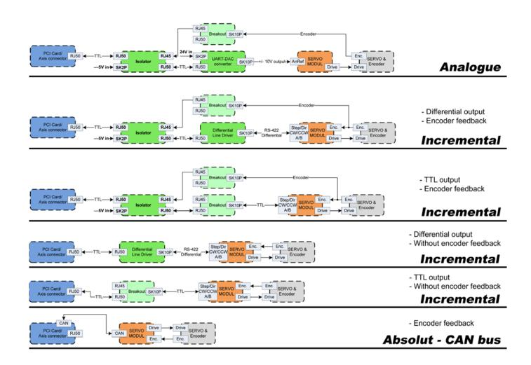
Figure 27.4: Servo axis interfaces
