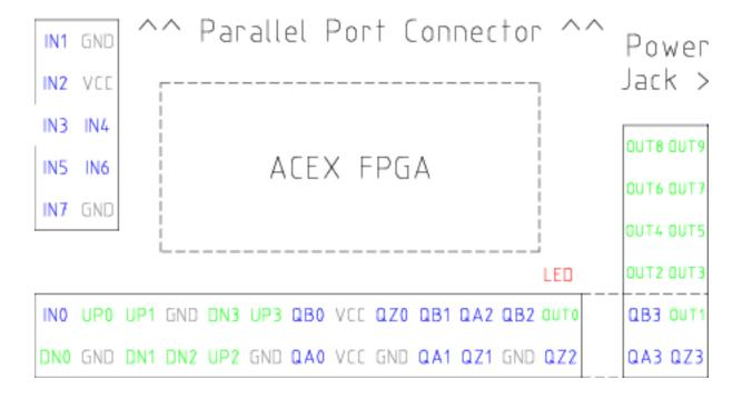
Figure 24.1: Pluto-Servo Pinout
