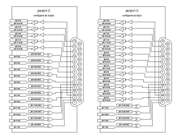
Figure 17.1: Parport Block Diagram
