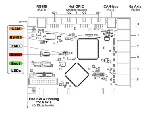
Figure 27.1: GM6-PCI card connectors and LEDs
