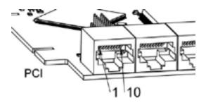
Figure 27.3: Pin numbering of axis connectors
