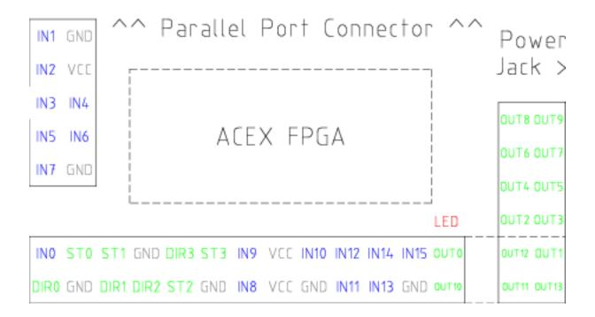
Figure 24.2: Pluto-Step Pinout
