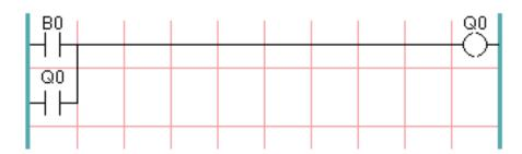
As before, when the user presses pushbutton B0, coil Q0 comes on. And when coil Q0 comes on, switch Q0 comes on. Now the interesting part happens. When the user releases pushbutton B0, coil Q0 does not stop as it did before. This is because switch Q0 of this circuit is effectively holding the user's pushbutton pressed. So we see that switch Q0 is still holding coil Q0 on after the *start* pushbutton has been released.
