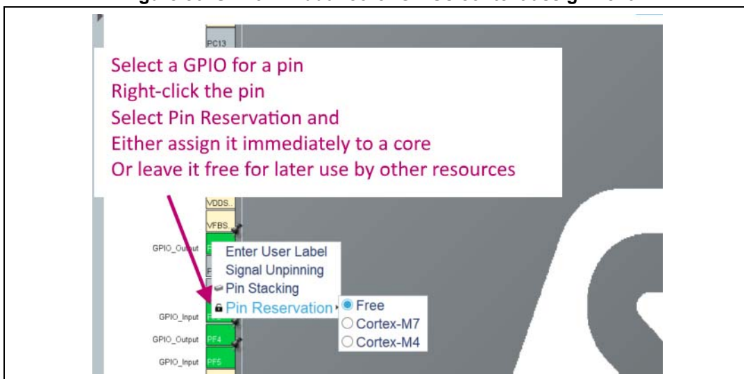
Figure 86. STM32H7 dual-core: GPIOs context assignment
