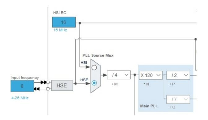
PLLCLK should be selected as system clock source and SYSCLK should show as 120Mhz.
