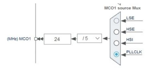
Choose PLLCLK to monitor the system clock rate. You need to divide by 4 or 5 to meet the max frequency of the output pin.
