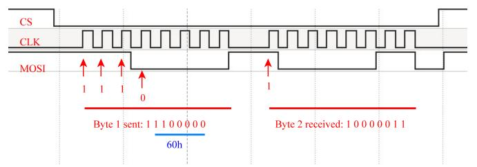
The first bit sent is a one, thus this is a read request going to the magnitometer asking for the value in register 60h which is named CFG\_REG\_A. The second data byte, 83h, is coming from the magnitometer and happens to be a value that was previously written to the register (the value in register 60h was 00h initially).
