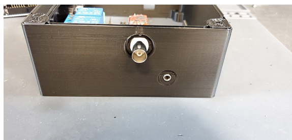
Fig. 70. Placement of BNC and 3.5 mm jack in housing skirt.
