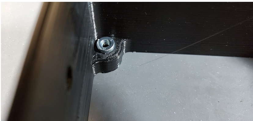
Fig. 64. Pushnut placement (not properly sunk).
