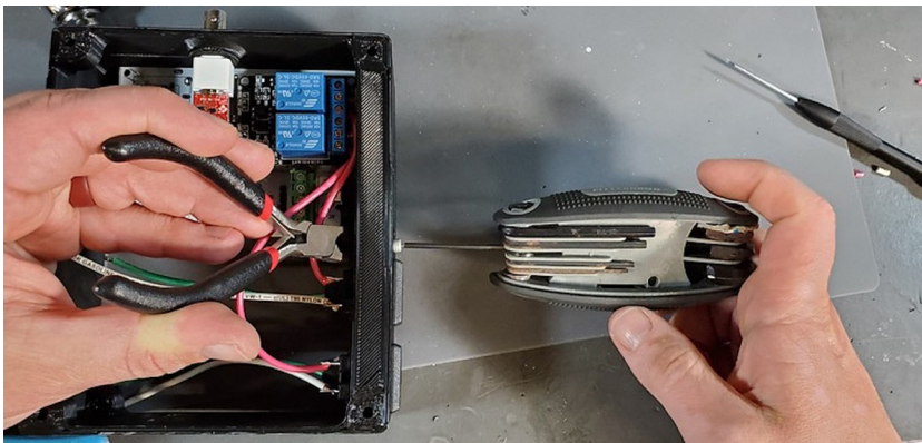
Fig. 71. Attach AC power receptacle to housing skirt.
