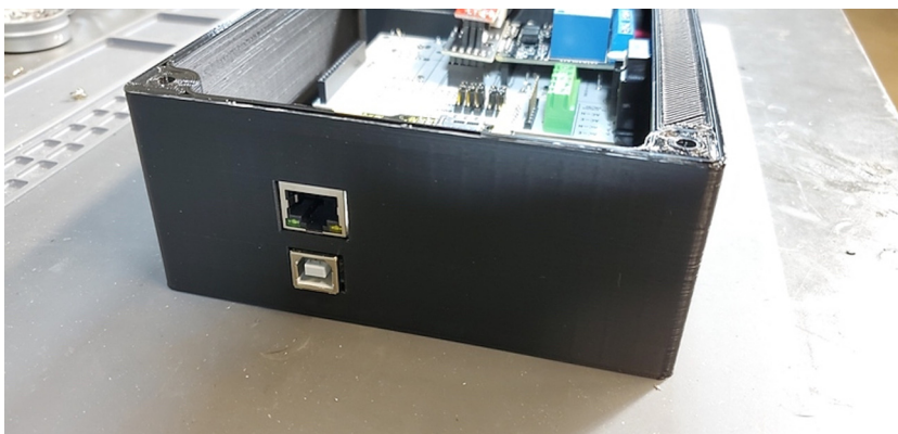
Fig. 75. Ethernet and USB outlet placement.
