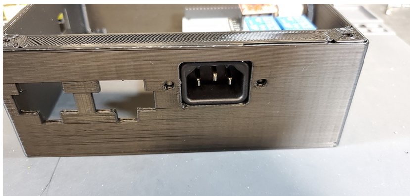
Fig. 69. Placement of electrical input in housing skirt.
