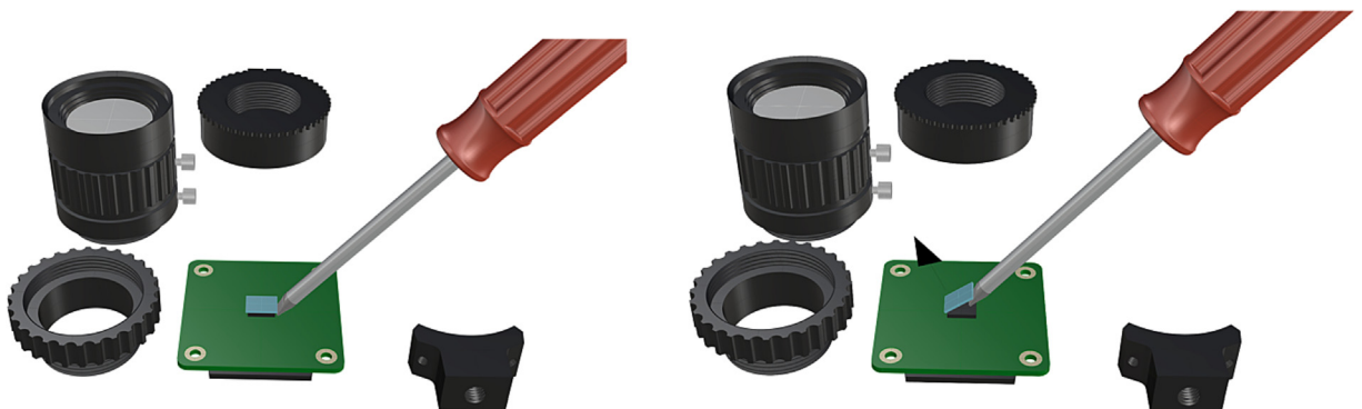
Fig. 22. A flathead screwdriver can be used to remove the FR filter from the Sony IMX477 sensor, removal of the IR filter exposing the sensor.
