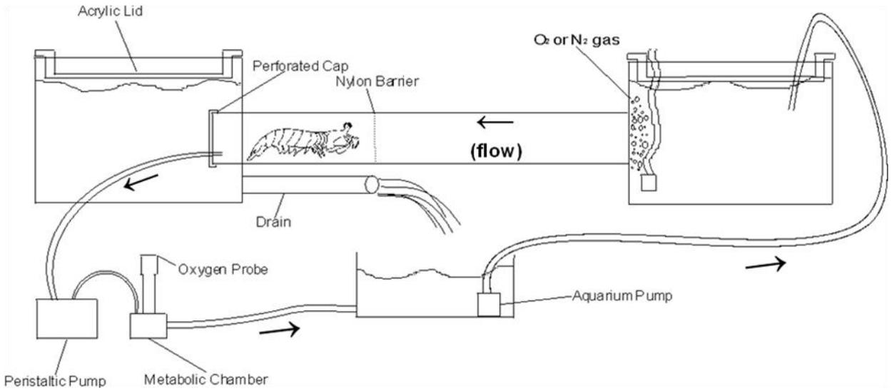
Figure 1. Experimental chamber. Circulation achieved via an aquarium pump.
