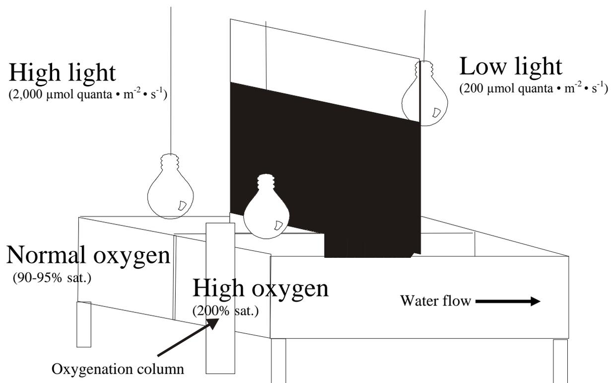
**Figure 3.** Diagram of the experimental setup. The oxygenation column oxygenated the incoming water for the high oxygen tank, while the normal oxygen tank received plain seawater. The divider between the high light and low light treatments extended down into the tanks, ending at the water level. Seawater flow passed from the high light ends of the tanks to the low light ends and exited via drains.
