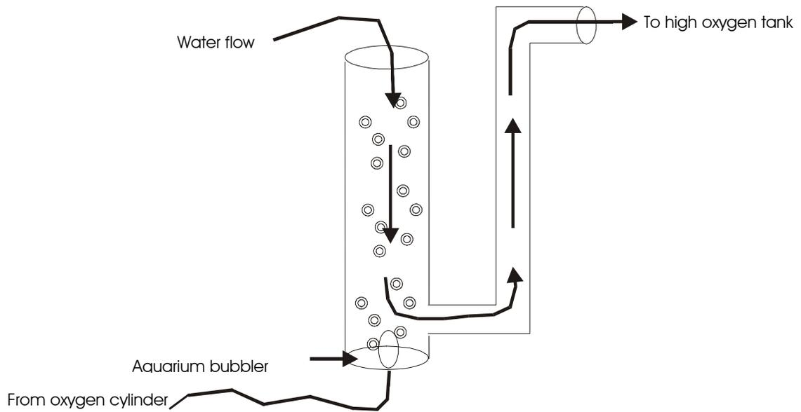
**Figure 2.** Diagram of the oxygenation column. Seawater flowed through the column, past the aquarium bubbler, and into the high oxygen tank. The bubbler was attached to an oxygen cylinder and bubbled pure oxygen through the column.
